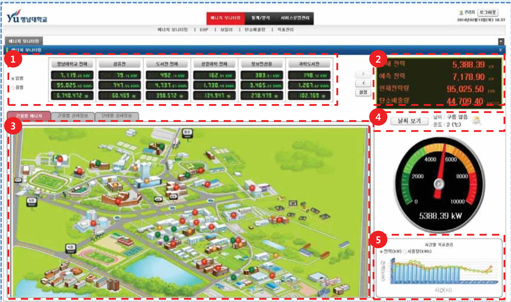
1) energy usage display, 2) peak electricity, 3) energy use state of each building 4) outdoor air information, 5) electric power usage and peak load
