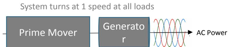
The Synchronous 'Fixed Speed' Generator
