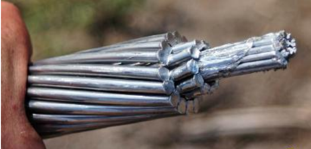
Figure 2: Aluminum conductor, composite reinforced metal matrix core (ACCR)
