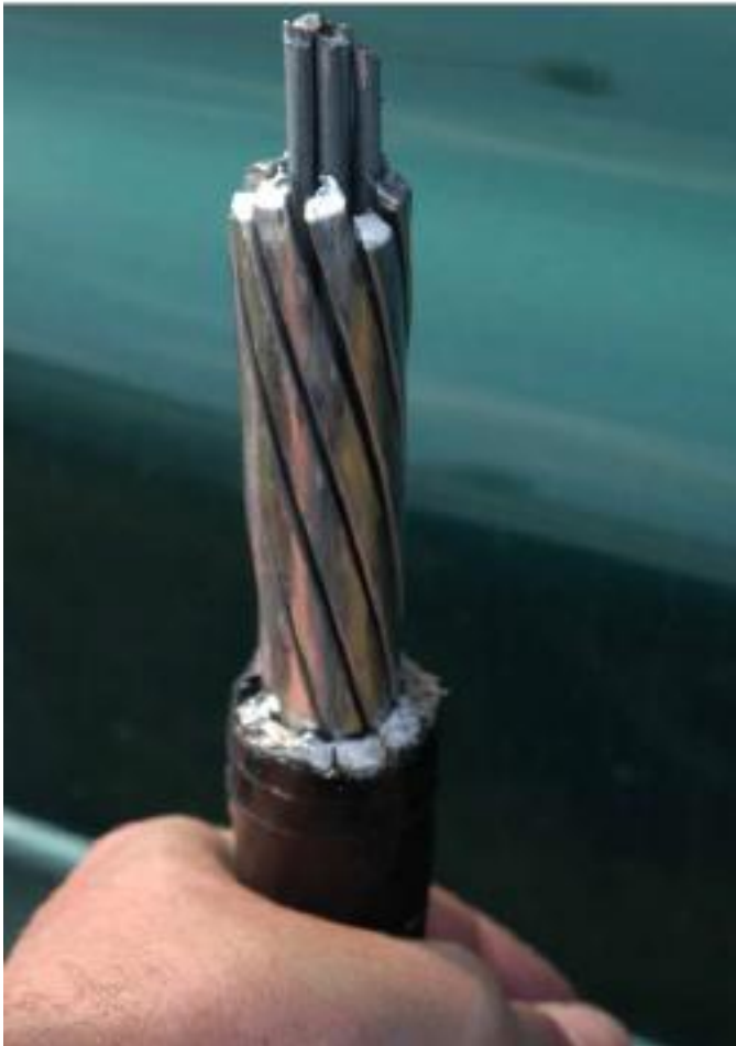
Figure 3: Aluminum conductor steel supported / trapezoidal wire (ACSS/TW)
