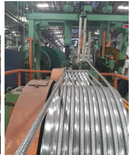
Manufacturing of ACCC/TW Dublin at Tenaga Cable Industry (TCI) in Malaysia (Carbon composite core from USA)
