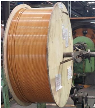
Manufacturing of ACCC/TW Dublin at Tenaga Cable Industry (TCI) in Malaysia (Carbon composite core from USA)
