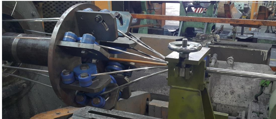
Manufacturing of ACCC/TW Dublin at Tenaga Cable Industry (TCI) in Malaysia (Carbon composite core from USA)
