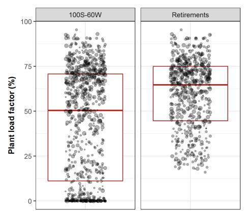
Change in coal plant load factors after 46 GW of coal plants are retired
