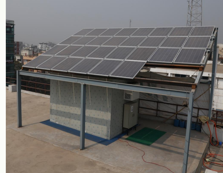
Fig. 3: Fabricated Solar PV-based cold storage being tested at UIU Lab, Dhanmandi, Dhaka.
