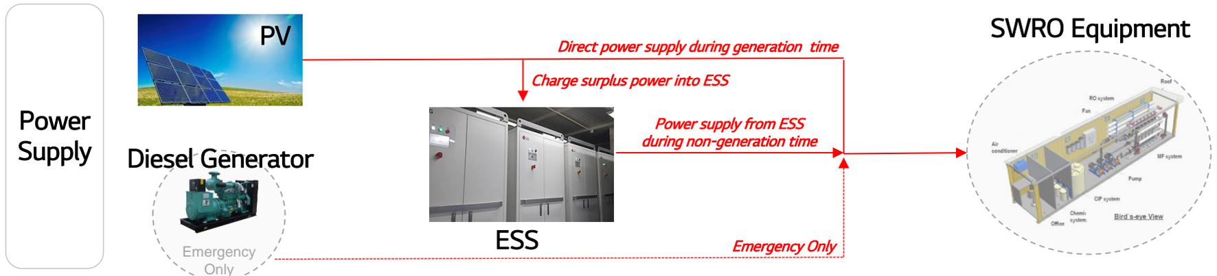
1) PV : Photovoltaic, 2) ESS : energy Storage System 3) MF : pretreatment(Microfiltration/Ultrafiltration) by Dual Media Filter 4) RO : Reverse Osmosis
