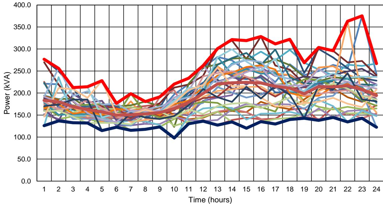
*Production (Load) profiles gathered during the field survey and referring to July 2016 (red tick line: highest hourly production profile; blue tick line: lowest hourly production profile; orange tick line: average hourly production profile).*
