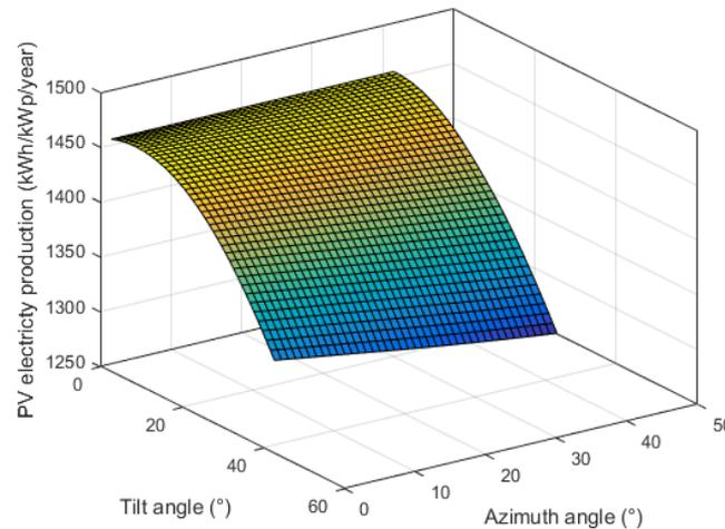
PV electricity production is in the range of 1.45-1.30 kWh/kWp.
