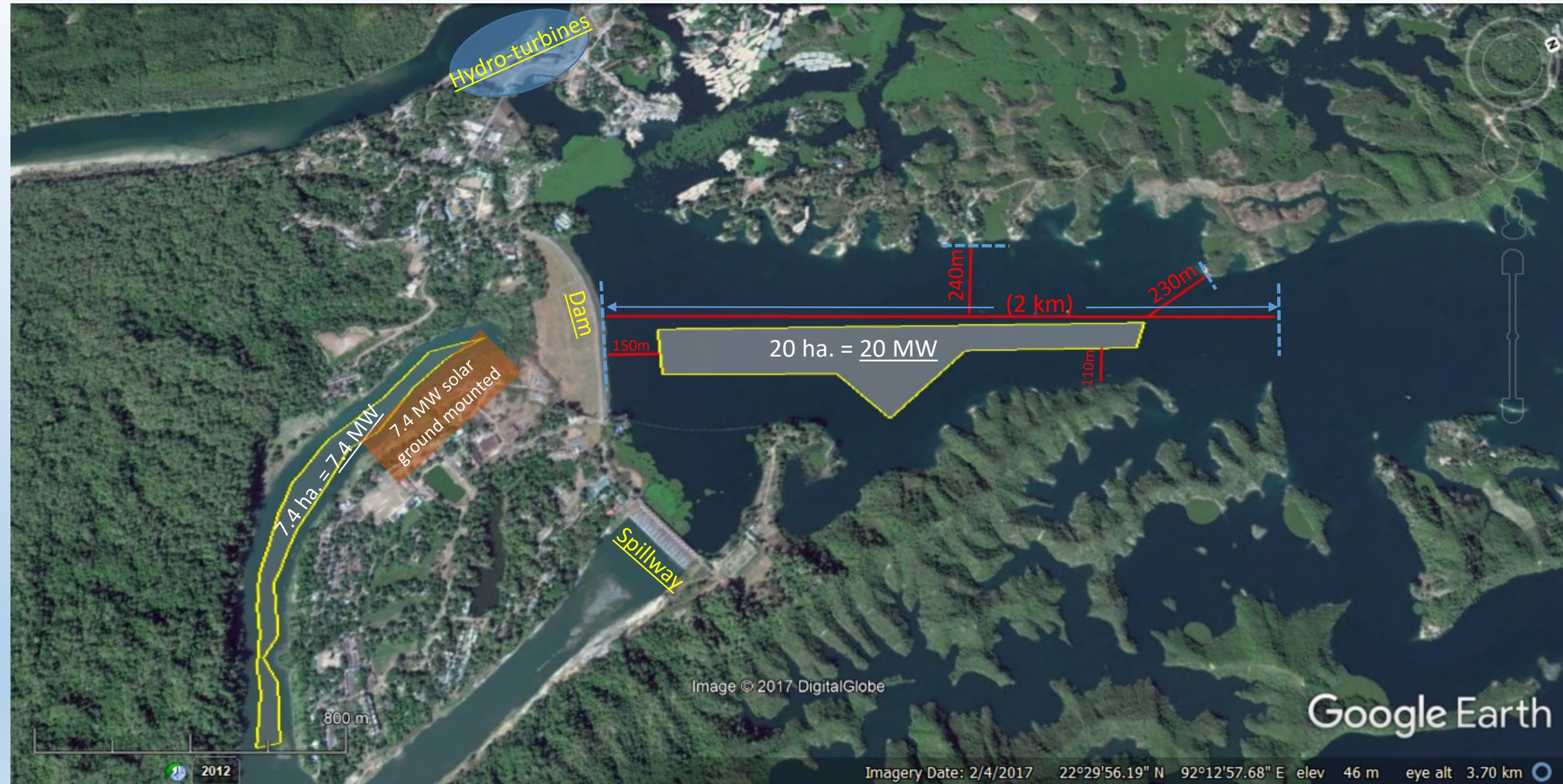
Site 1: 7.4 MW floating solar PV placement adjacent to 7.4 MW ground mounted solar PV
