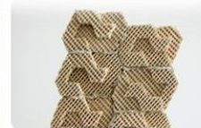
The 3D-printed cool brick can hold water in its pores, like a sponge. Design studio Emergingobjects has come up with a simple way to cool homes, build them with 3D-printed porous bricks called Cool Bricks which can be filled with water to bring down temperatures.
