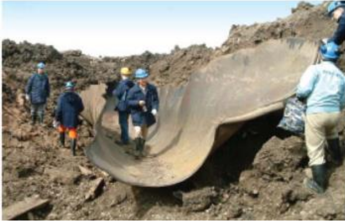
A running fracture-result of a test
