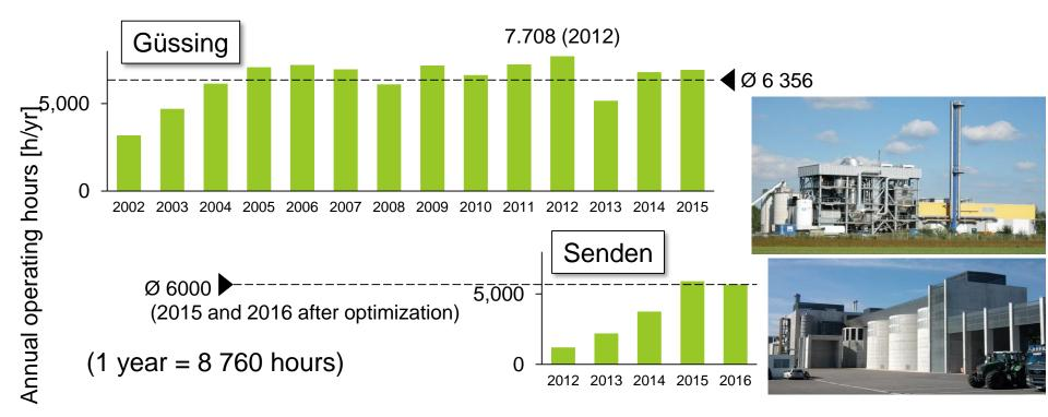
Güssing: 8 MW fuel input $\rightarrow$ 2 MW power + 4.5 MW heat Senden:14.3MW fuel input $\rightarrow$ 5 MW power + 6.5 MW heat
