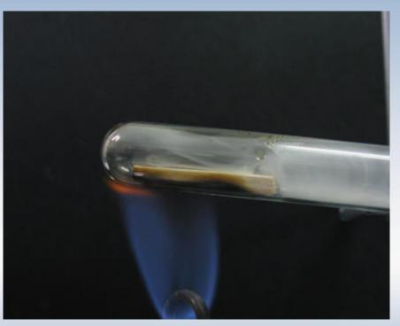
Combustion:  $C_xH_yO_z+a_sO_2 \rightarrow xCO_2+(y/2)H_2O+heat$
