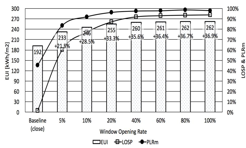
Natural Ventilation Model: EnergyPlus "Zone Ventilation: Wind and Stack Open Area"
