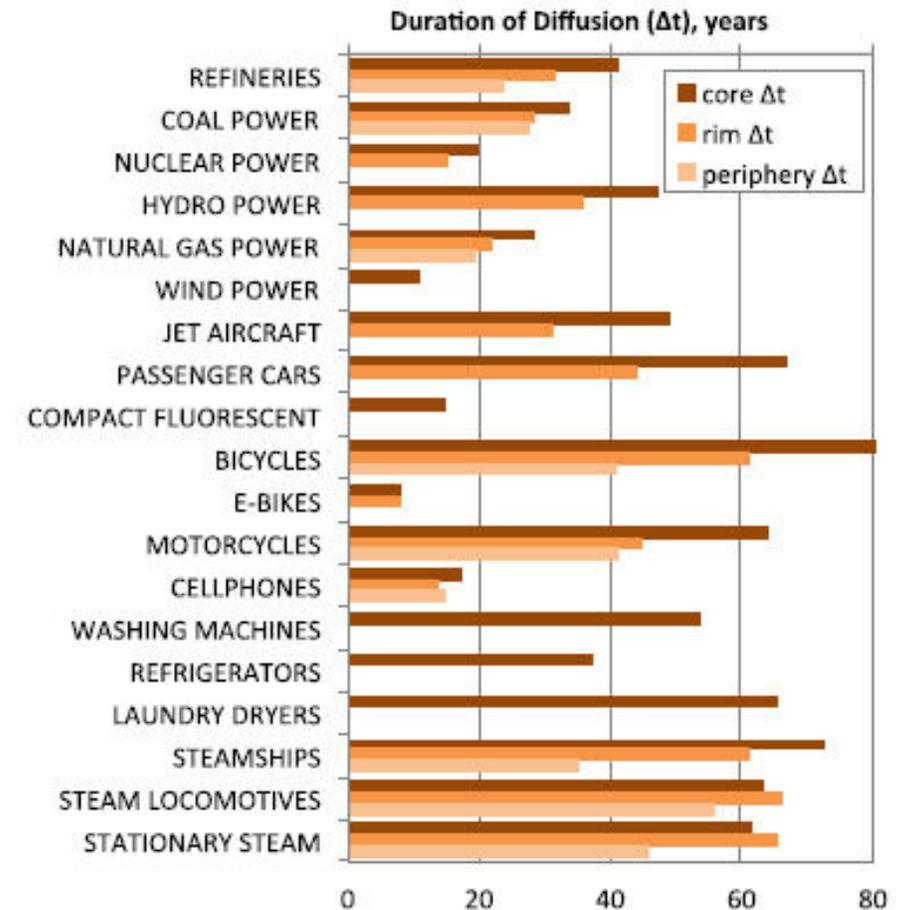
**Fig. 2.** Diffusion speeds accelerate as technologies diffuse spatially. Notes: Bars show durations of diffusion measured by cumulative total capacity installed, with historical data fitted via a logistic growth curve and the diffusion duration expressed as  $\Delta t$  in years. 'Core' is typically within the OECD; 'Rim' is typically Asian countries; 'Periphery' is typically other world regions. For details and data, see: [42,3].
