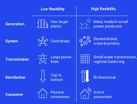
Flexibility creates system value through reduced build-out needs while operating and decarbonising the system more efficiently
