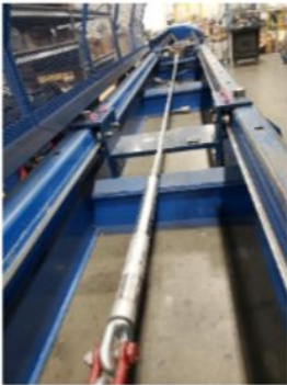
Figure 1 – Tensile load test setup for complete conductor.
