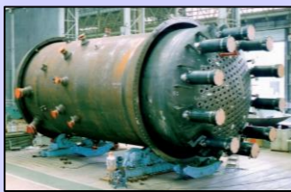
Reactor Pressure Vessel
